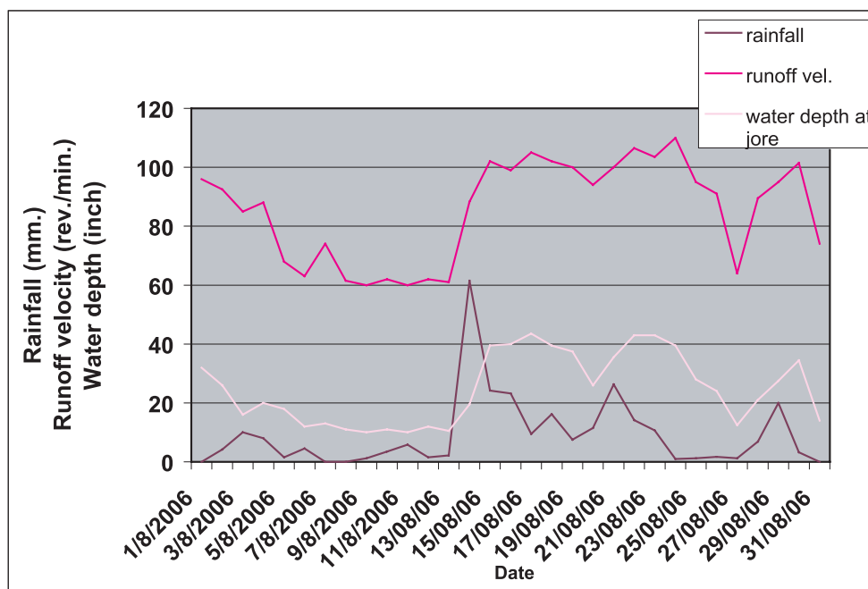
Graph 2.5.6 Correlation between rainfall, run-off velocity and water-depth at 'jore' (rivulet)
